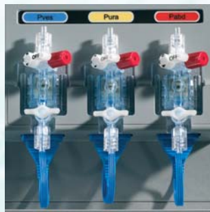
Pressure transducer Several options - As shown, Medex Dome system or Micro-tip catheter.
