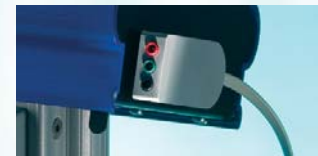
EMG Compact EMG preamplifier measures pelvic floor activity.
